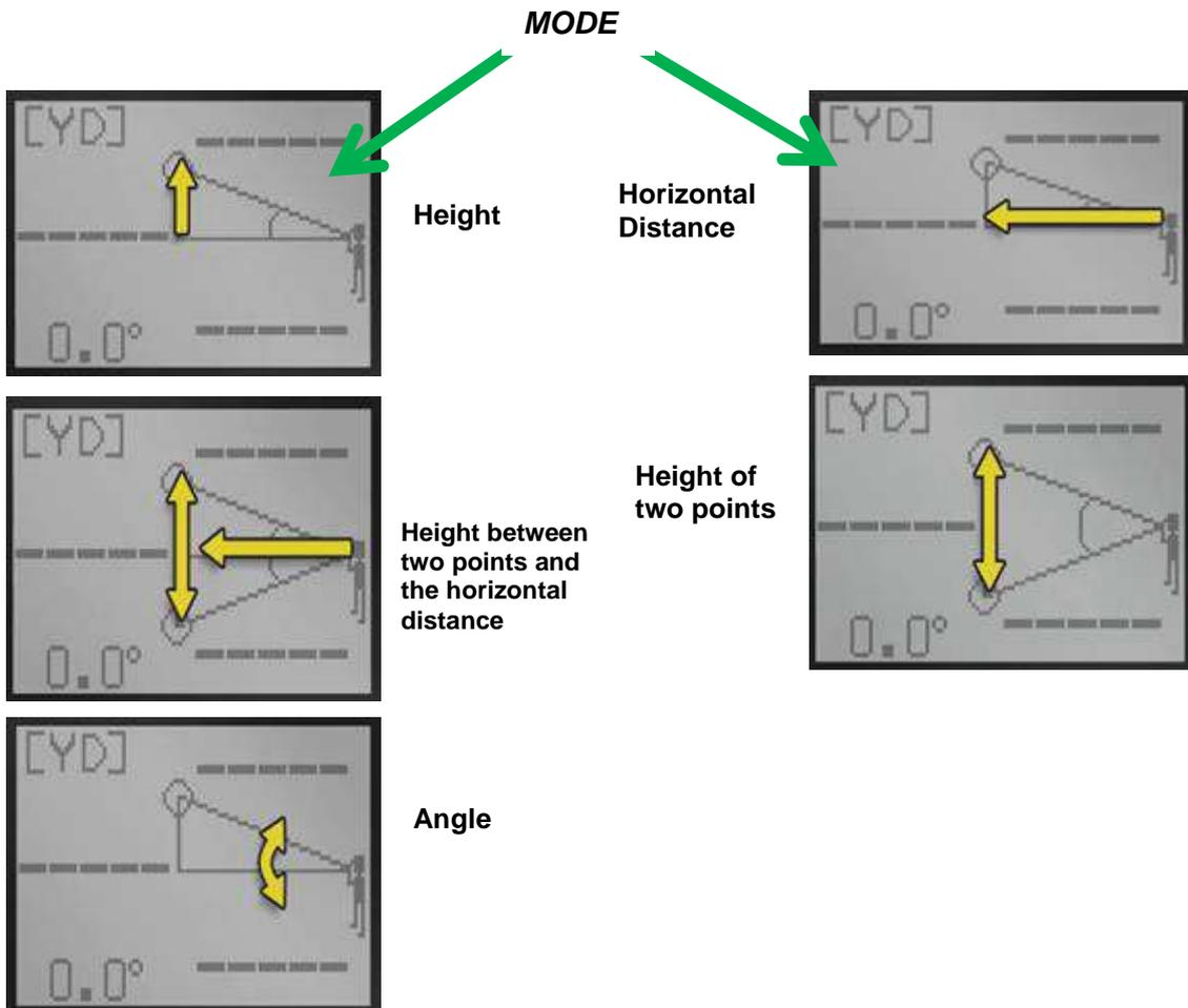
2. To change the **Units of Measurement** (metres [M], feet [FT]) from the default **[YD]** or from other unit that you are not going to use, press and hold the **MODE** button for a couple of seconds and internal display will change to the new priority mode. Press and hold again and again until you have reached the unit you are going to use.
