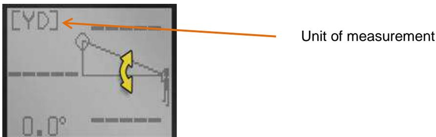
3. **Priority Mode** - set this when the object you are trying to measure is behind another object. In our case a tree is blocked by a patch of other vegetation
