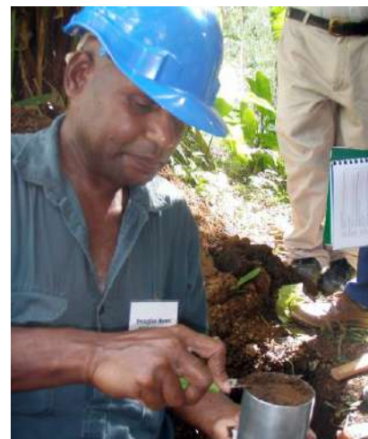
Figure 2. The Rowfit sampler is designed to take an undisturbed core 10 cm deep from stone-free or slightly stony soils. It consists of a stainless steel outer cylinder which encloses a removable aluminium liner. From top left: gently hammering the sampler into the soil using a rubber mallet; extracting the sampler; unscrewing the top; cutting excess sample from the base of the extracted internal liner of the sampler before bagging the sample.
