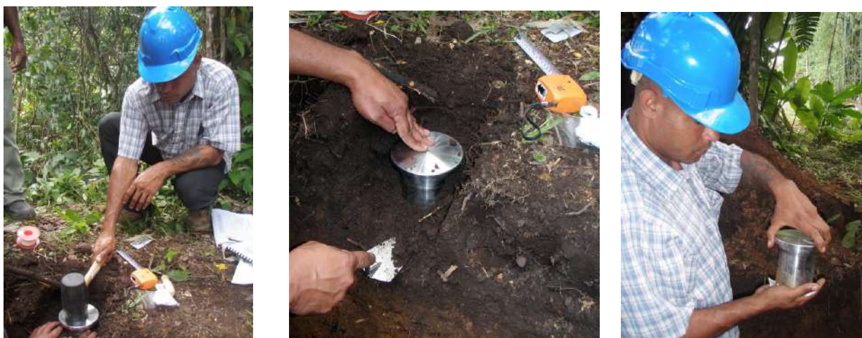
Figure 2. The Rowfit sampler is designed to take an undisturbed core 10 cm deep from stone-free or slightly stony soils. It consists of a stainless steel outer cylinder which encloses a removable aluminium liner. From top left: gently hammering the sampler into the soil using a rubber mallet; extracting the sampler; unscrewing the top; cutting excess sample from the base of the extracted internal liner of the sampler before bagging the sample.
